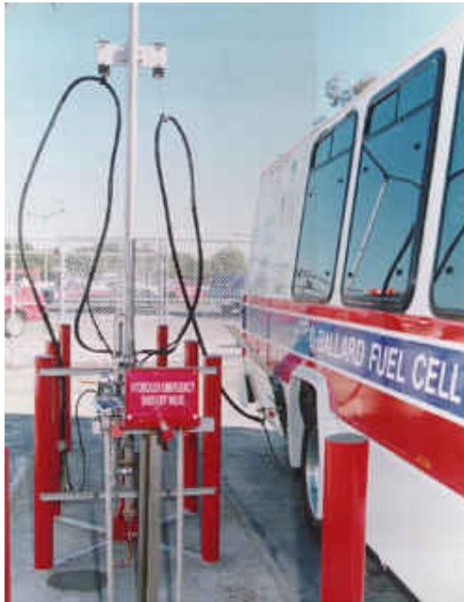
Picture 7.2: Refueling the Ballard Fuel Cell Bus at the CAN Solar Hydrogen Refueling Station
